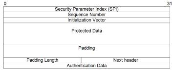
Figure 3 - Encapsulating Security Payload
